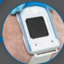
Visually confirm complete contact with skin by all the microblister holes in the Harvester, and reposition if necessary
