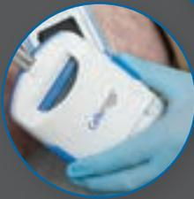
Unlatch the Vacuum Head from the Harvester by squeezing the blue handle on either side of the Vacuum Head
